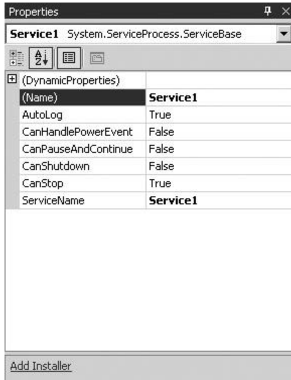
Figure 12.10: The Properties window for a service project, showing the Add Installer link.
